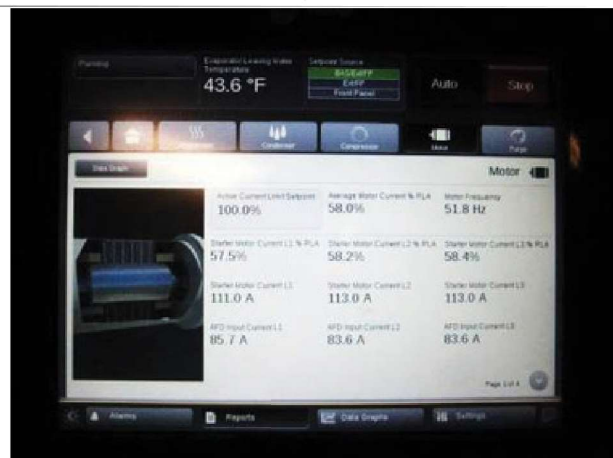
Chiller capacity limit is set at 100%. A lower setpoint should be received/considered for electrical demand savings. Typical capacity during significant load conditions is less than 60% as indicated above (57.5%)
