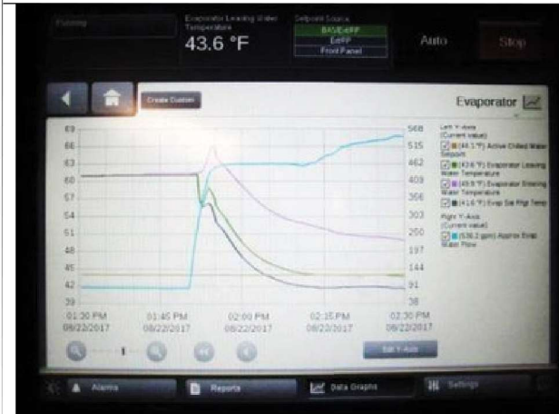
Chiller came back on line at 1:50pm, OFF for over 2 hours, and required nearly full capacity to recover while increasing building electrical peak demand.
